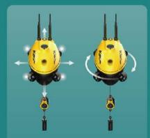
CHASING F1 has a vector layout propulsion system with four thrusters, which can achieve multiple-freedom motion. The all-directional horizontal movements controlled through APP make finding fish faster and more accurately.
